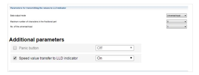
Data Mode, select the data source that should be used to display values on the Omnicomm LLD indicator.
