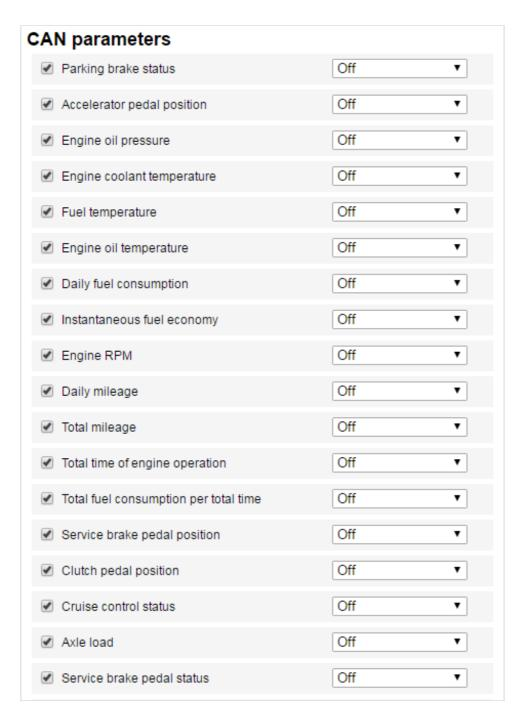
Refer to the list and select the parameters whose values you need to display in Omnicomm Online by ticking the box in the 'Use' column appropriately. If you need to add parameter readings from the CAN bus that are missing from this list, go to Omnicomm Configurator and click on 'Add'. You will be taken to the following screen:
