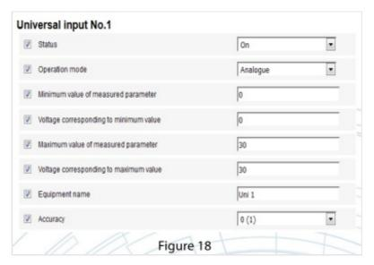
Universal input type is determined automatically depending on the additional equipment connected to the uni- versal input (Figure 18). Enter the required settings depending on the universal input type according to the Omnicomm Configurator User Manual or Omnicomm Terminals Operating Manual.
