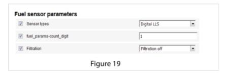
The type and number of LLS fuel level sensors are determined automatically and, if necessary, are available for change (Figure 19).
