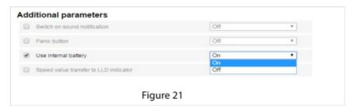
"Use internal battery" — select on/off to activate or deactivate use of the internal battery when the main power is off and Omnicomm Profi terminal operates in the mode "Collect data at jolting" (Figure 21).
