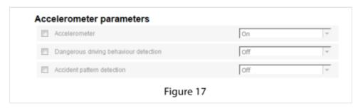
"Accelerometer" — select on/off to activate or deactivate measurement of VH acceleration. "Dangerous driving behaviour detection" — select on/off to activate or deactivate detection of dangerous driv - ing behaviour when the set threshold values are exceeded. When the dangerous driving behaviour detection is on:
