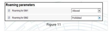
"Roaming parameters" — select SIM-card option to operate in roaming. Possible options are "Allowed", "Prohib- ited" (Figure 11).
