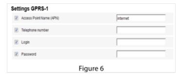
"Access Point Name (APN)" — enter GPRS access point name (Figure 6). The GPRS access point name for operators can be obtained from the mobile operator whose SIM-card is installed in the terminal. "Telephone number" — number of the SIM-card installed in the terminal. "Login (APN)" and "Password (APN)" — if necessary, enter the login and password to access the point APN. A login and a password are supplied together with the SIM-card of the mobile operator.
