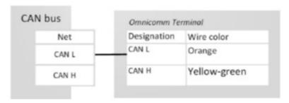
Configuring the reception of data on the fuel volume in the tank from the vehicle CAN bus Connect and configure reception of the vehicle equipment operation parameters from CAN J1939 data bus and set the setting of fuel sensor – "CAN Sensor".
