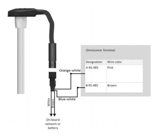
Connect Omnicomm LLS-AF fuel level sensor according to the diagram:
