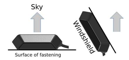
We recommend to install it on the windshield or on the horizontal surface of the instrument panel in a place providing a good radio pick-up range of the sky.
