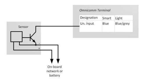
Connect contact sensor according to the diagram:
