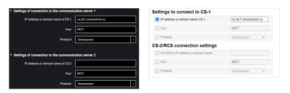
"IP address or domain name of CS 1" – enter IP address or domain name of the communication server: cs.dc1.omnicomm.ru.
