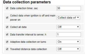
"Data collection timer" – set the value of the period of Terminal requesting modules and external devices connected to it. Default value - 15 seconds. Value range - from 1 to 240 seconds (except for Smart). Value range for Smart - from 15 to 240 seconds.
