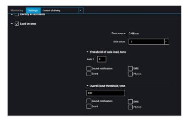
"Data source" displays the axle load data source. Possible options: ALM Weight Indicator and CAN.
