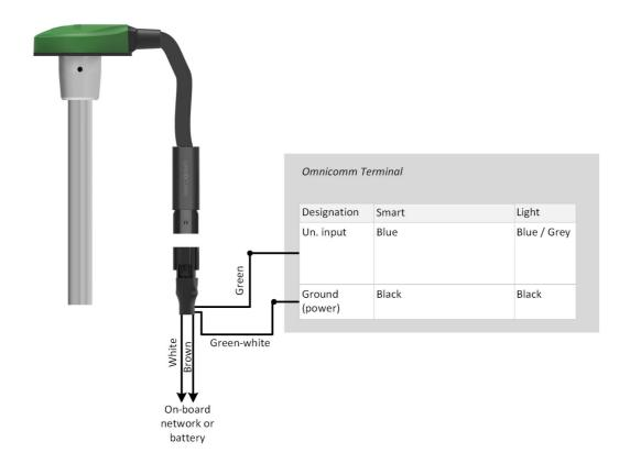
Connect several Omnicomm LLS-AF sensors to the Light terminal one by one, starting with 1 universal input.
