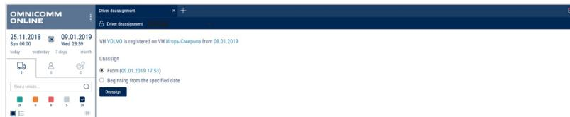
Select the today's date or select any past date and time from which it is required to finish the driver assignment to the VH.
