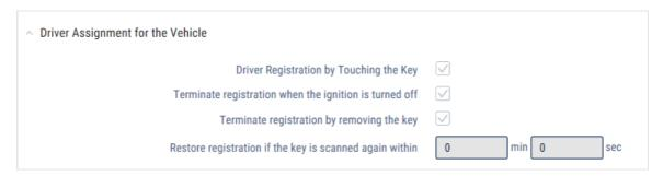
"Driver registration by touching the key" – y- check the box to sign in a driver when an RFID card or an iButton key is scanned.
