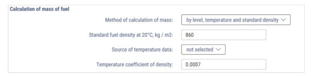
"Fuel rated density at 20°C, kg/m³" - enter the rated density of the fuel. Default value - 860, kg/m³
