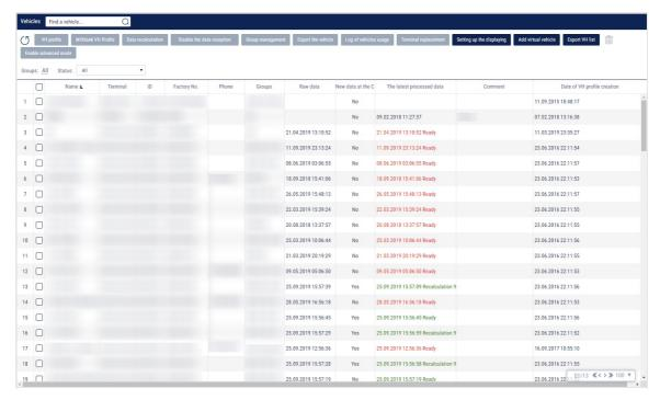
"Raw data" displays the date and time of receipt of the latest data from the communication server for each vehicle.
