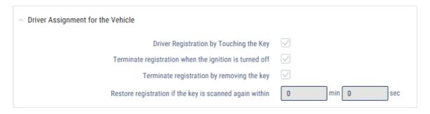
"Driver sign in by tag reading" – y- check the box to sign in a driver when an RFID card or an iButton key is scanned.
