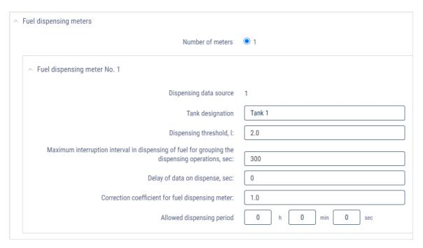
"Tank designation" – select for which tanks this meter is used to track the dispensing operations.
