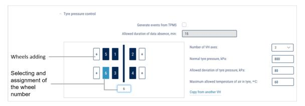
"Generate events from TPMS" – check the box to process data from the tire pressure monitoring system.
