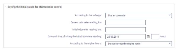
"Initial odometer reading, km" – enter the mileage reading from the odometer.
