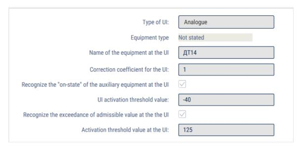
**"Equipment name at universal input"** – enter the name of the sensor or the name of the measured value.
