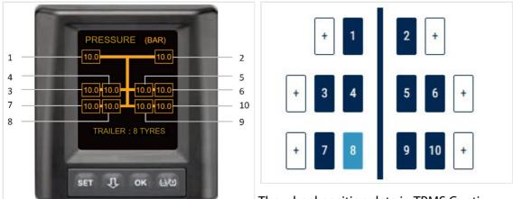
The wheel position data in TPMS Conti Pressure Check is transmitted in CAN J1939
