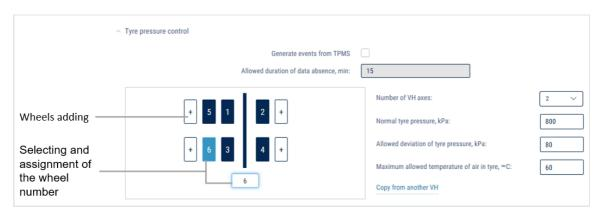
"Create events from TPMS" – check the box to process data from the tire pressure monitoring system.
