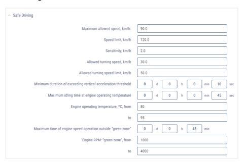
"Maximum allowed speed, km/h" – the value of the vehicle speed, above which Omnicomm will register vehicle movement as exceeding the maximum allowed speed. Possible values: from 0 to 300 km/h. Default value - 0 km/h (no violations will be recorded).
