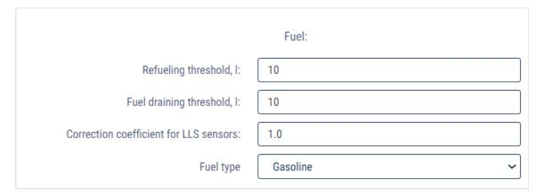
"Refueling threshold, I" (from 0 to 28000) - the amount of fuel to which the total amount of the vehicle's fuel must be increased during the designated period of time, in order for the refueling to be registered.
