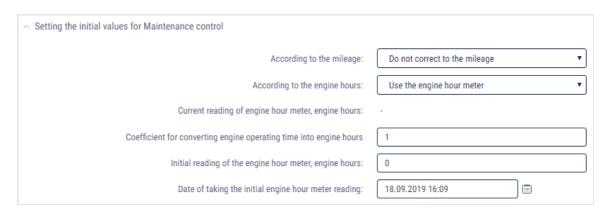
"Coefficient for converting engine operating time into engine hours" - specify the conversion coefficient of the engine operation time to engine hours, indicated in the vehicle documentation.
