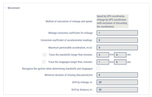
"Method of calculation of mileage and speed" allows you to choose based on what data and using which method are the mileage and speed calculated. Possible options:
