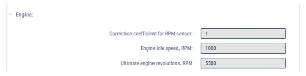
"Correction coefficient for the RPM sensor" – the coefficient of conversion of the number of pulses recorded by the RPM sensor into the number of revolutions.
