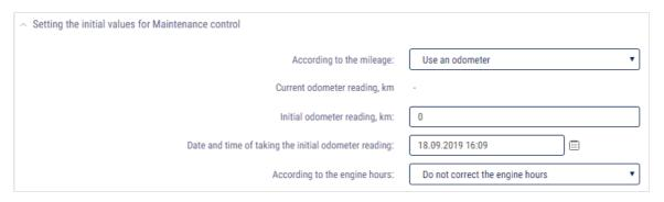
"Initial odometer reading, km" – enter the mileage reading from the odometer.
