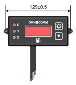
While installing the Omnicomm LLD fuel volume indicator with the help of self-tapping screws, drill two 2.5 mm diameter fixation holes according to the installation dimensions.
