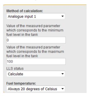
"Value of the measured parameter that corresponds to the minimum fuel level in the tank" — enter the value (in Volts) from the calibration table of the analogue sensor that corresponds to an empty tank.
