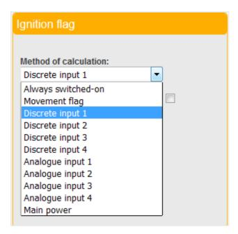
Select the parameter, based on which Omnicomm Online software will record the event of VH ignition as on/off.
