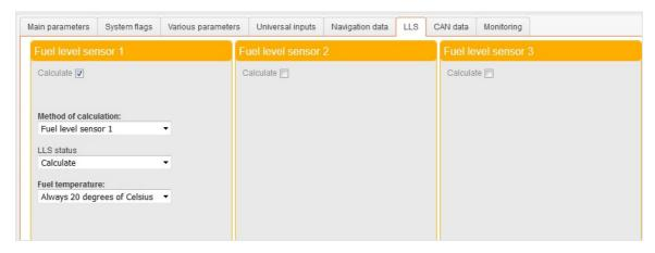
In the field "Method of calculation", select the parameter based on which Omnicomm Online software will record the fuel level.
