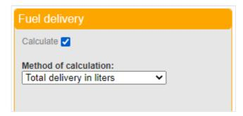
In the "Calculation method" field, select the parameter which Omnicomm Online will use to calculate fuel dispensing.
