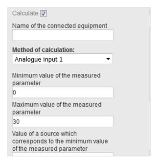
"Minimum value of the measured parameter" set the minimum value of the parameter measured by the sensor. The parameter is measured in appropriate units of measurement, e.g. for temperature – in degrees Celsius.
