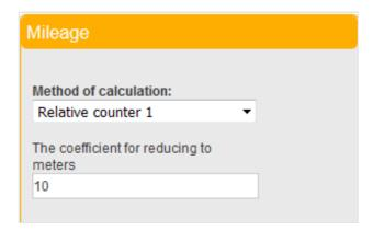
"The coefficient for reducing to metres" — enter the factor to multiply the mileage received by, from the absolute counter in order to convert the mileage value to metres.
