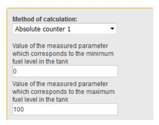
"Value of the measured parameter that corresponds to the minimum fuel level in the tank" — enter the value (in Hertz) from the calibration table of the fuel level sensor connected to the third-party terminal that corresponds to an empty tank.
