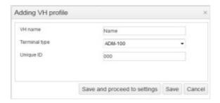
Enter the name and registration number of the VH next to "**VH Name**". The VH name must contain 3-64 characters. It should coincide with the VH name loaded in Omnicomm software.
