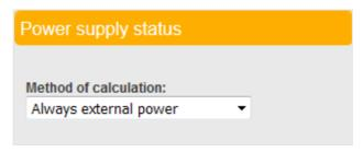
In the field "Method of calculation", select the parameter based on which Omnicomm Online software will record the terminal's power supply status.
