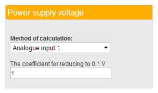
"The coefficient for reducing to 0.1 V"- enter the factor by which to multiply the received power supply voltage value to convert it to dimensions of 0.1 V;
