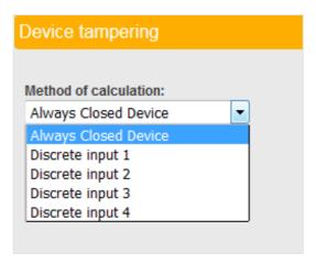
In the field "Method of calculation", select the parameter based on which Omnicomm Online software will record terminal tampering.
