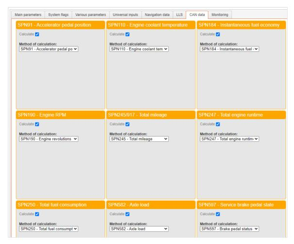
In the field "Method of calculation", select the parameter based on which Omnicomm Online software will record the CAN parameter.
