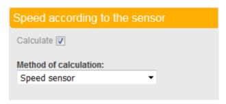
In the field "Method of calculation", select the parameter based on which Omnicomm Online software will calculate the VH speed.
