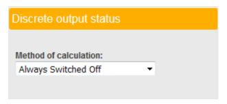
In the field "Method of calculation", select the parameter based on which Omnicomm Online software will record the discrete output status.
