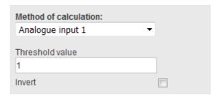
• "Main power". This Method of calculation is set up if the third-party terminal transmits data about main power availability. Omnicomm Online software will record ignition on when the VH onboard power network voltage exceeds "Threshold value".
