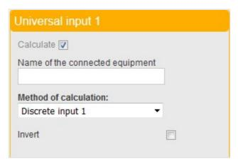
"Calculate" — tick if it is required to control the universal input.
