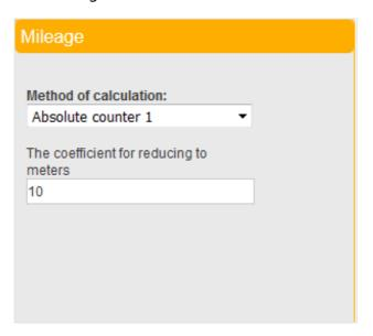
"The coefficient for reducing to meters" — enter the factor to multiply the mileage received by, from the absolute counter in order to convert the mileage value to metres.
